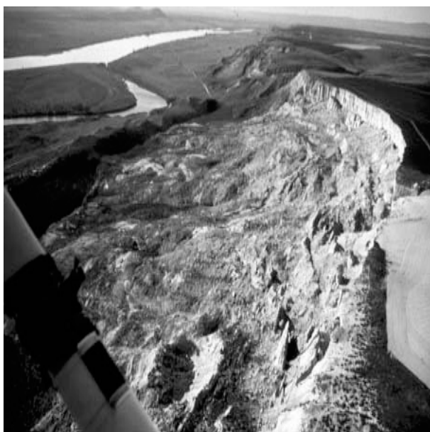
Figure 3G April 1981 aerial oblique view of the 12-million-m 3 , irrigation-induced Savage Island landslide on the Columbia River, south-central Washington State, U.S.A. In the spring of 1981, hundreds of baby cliff swallows were killed when their nests in the 25-m-high main scarp were destroyed because of catastrophic headward recession of the landslide to the location shown.
