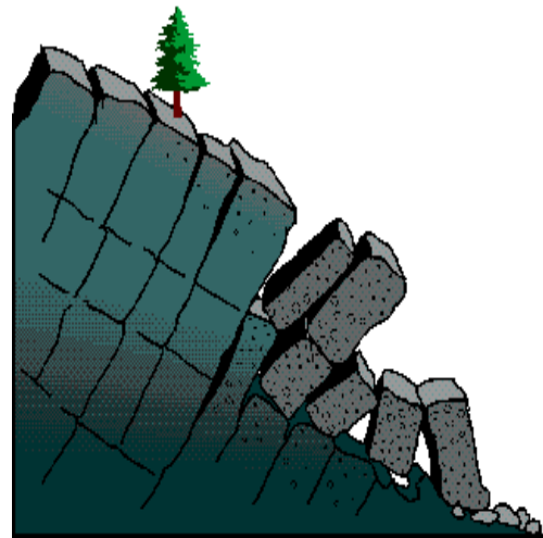
1E: Topple: the end-over-end motion of rock down a slope. (Source: http://pubs.usgs.gov/fs/2004/3072 ).
